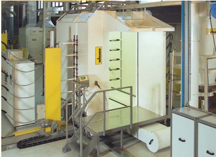
Fixed integral booth floor with blow-out device
